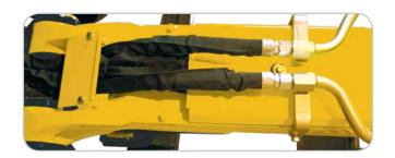
> Careful routing and protection of the hydraulic pipes on the boom and on the right side of the machine under the step. You can remove the step to access the sockets and change the equipment pipes.
