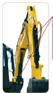
> Cylinders completely protected (rod and cylinder) by highly elastic steel plates to resist any possible shocks.
